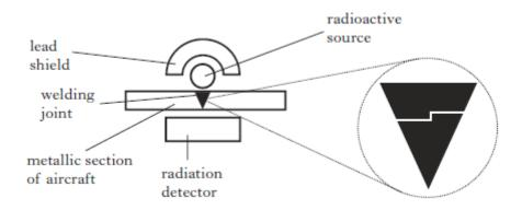
The radiation detector monitors the amount of radiation passing through the section of the aircraft being checked.
