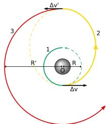
• Gravity Assist — rather than using fuel flight planners can use celestial object's gravity to add or remove orbital velocity (see below). This is needed for any mission beyond Jupiter!
