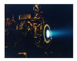
These engines accelerate ions in a electric field to generate thrust rather than using combustion. There are a lot of different types of ion thruster (such as Hall effect thrusters) but they all have similar properties. Ion thrusters produce very little force compared to a chemical rocket but they can produce force for a long time and use very little mass of 'fuel' to do so. This means that they are convenient for sending small probes and spacecraft on long missions.
