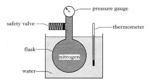
a) The pressure of the gas is 109kPa when its temperature of  $15^{\circ}$ C.
