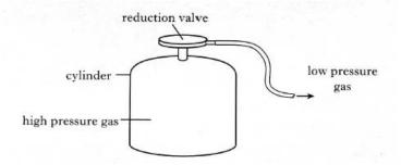
The pressure of the gas in the cylinder is  $2x10^6$ Pa. The pressure of the gas as it leaves the reduction value is  $4x10^5$ Pa.
