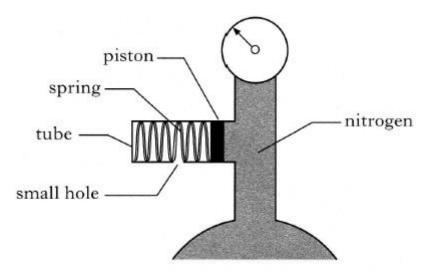
The piston of cross-sectional area **4x10<sup>-6</sup>m<sup>2</sup>** is attached to the spring.
