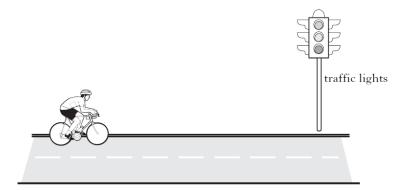
The cyclist approaches traffic lights at a speed of 8ms<sup>-1</sup>. He sees the traffic lights turn to red and 3 seconds later he applies the brakes. He comes to rest in a further 2.5 seconds.
