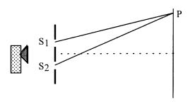
A microwave detector shows a minimum at P. P is the position of the first-order minimum, ie it is the second minimum from the centre.
