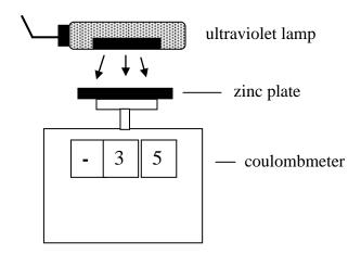
The threshold frequency of radiation for zinc is  $6.50 \times 10^{14}$  Hz.
