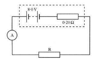
The reading on the ammeter is 4.0 A.
