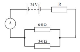
The reading on the ammeter is  $2 \cdot 0 A$ .
