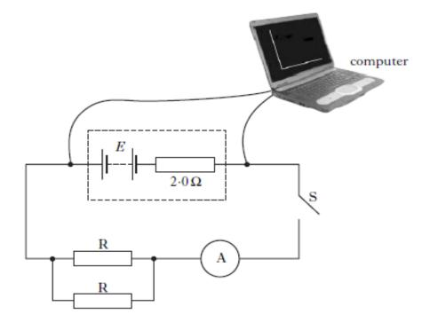
(c) Switch S is opened. A second identical resistor is now connected in parallel with R as shown.
